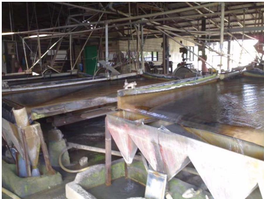
FIG. 17. Wet processing of amang.
