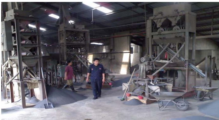
FIG. 18. Dry processing of amang.
